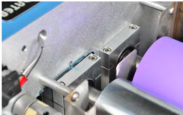
Fast and easy removal of applicator and metering rollers
